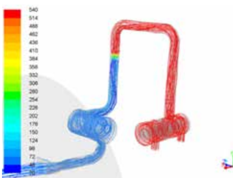
Flow pathlines through the exhaust gas system and colored by temperature
